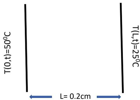
We will now break this plane wall into discrete sections of thickness  $\Delta x=0.02\text{ cm}$ .
