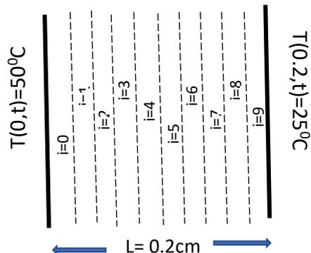
Now denote the leftmost element at  $x=0$  by  $i=0$ , the next element by  $i+1=1$  and so on. The rightmost element is denoted by  $i=n-1=9$ .
